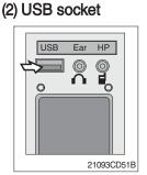
① This socket is used to charging the mobile phone.
