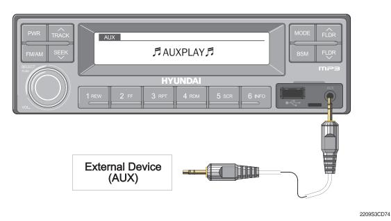
• Operates only when the external device is connected to the AUX interface. When an AUX device is connected to the system using an AUX cable, the system automatically switches to AUX mode.
